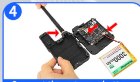
Connect the antenna, battery, and GPS
